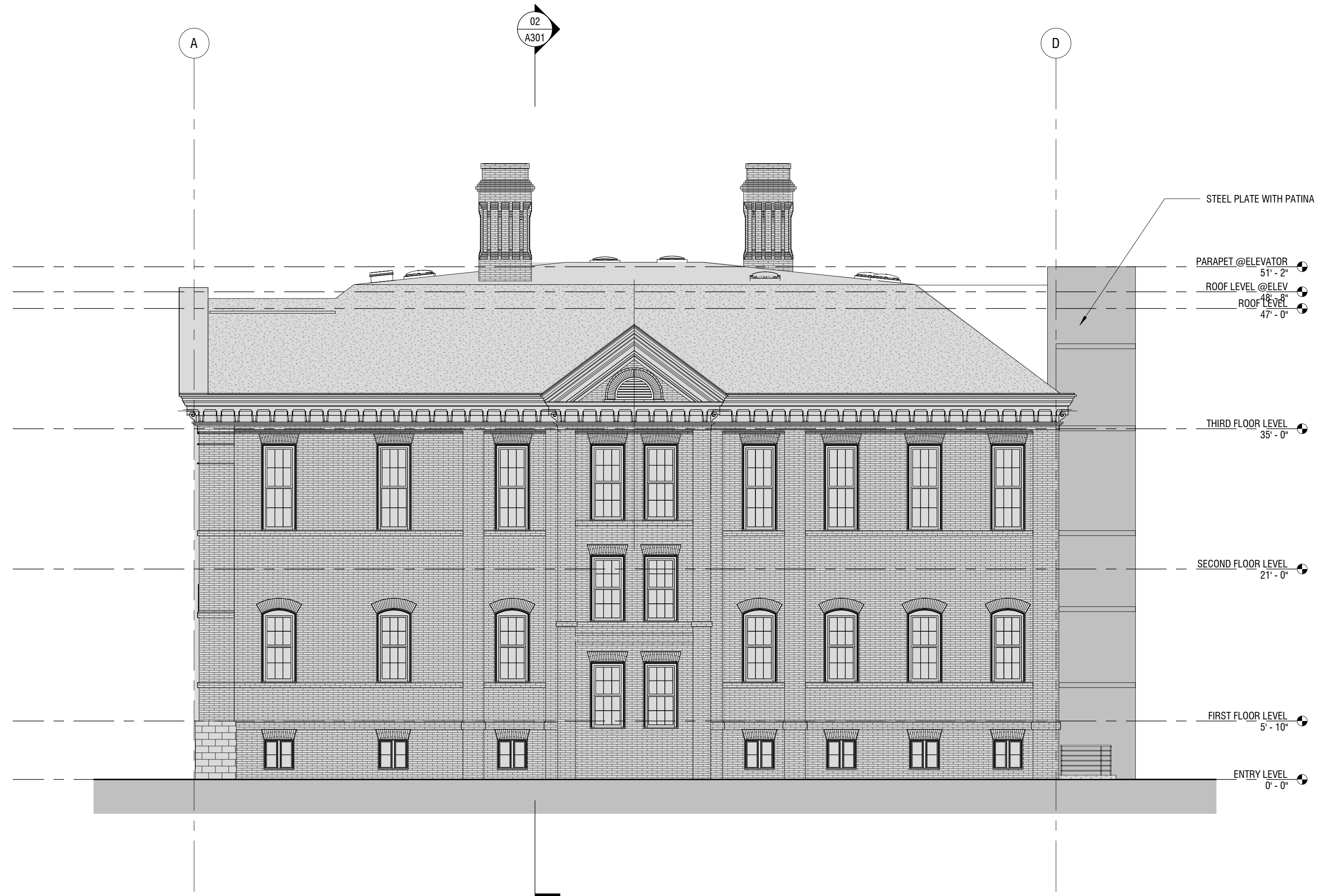
04 BUILDING ELEVATION WEST SCALE: 1/8" = 1'-0"
